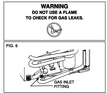
The gas supply system must incorporate a pressure regulator to maintain a supply pressure of not more than 13.5 inches water column, static (no load).
